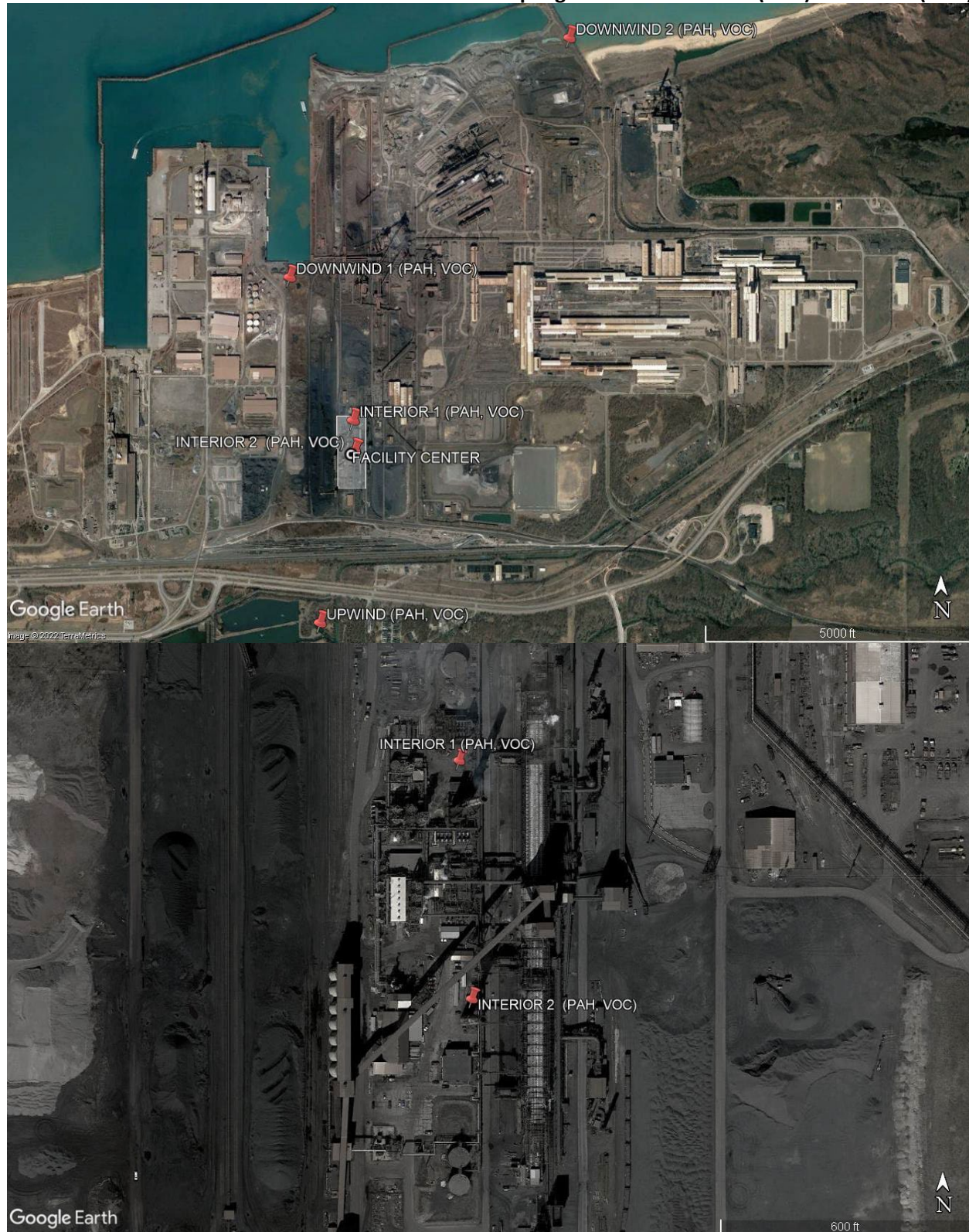
Figure 1-2: Cleveland-Cliffs Burns Harbor – Fenceline and Interior Sampling Locations – TO-13A (PAH) and TO-15 (VOC)
